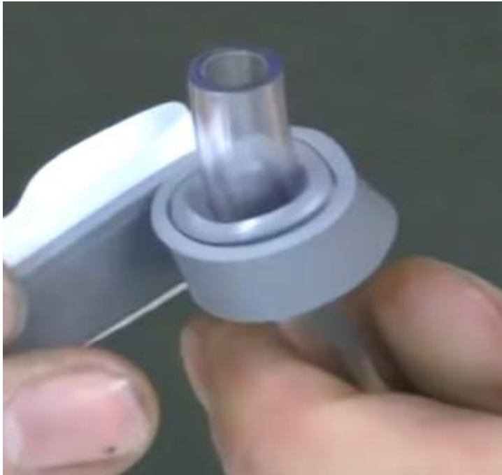
Figure 5. Gum tape applied to vacuum tubing.
